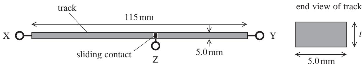
The length of the track is 115 mm and the width is 5.0 mm.
