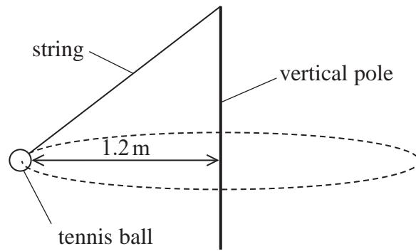
The radius of the path of the ball is 1.2 m and the speed of the ball is  $3.8 \text{ ms}^{-1}$ .
