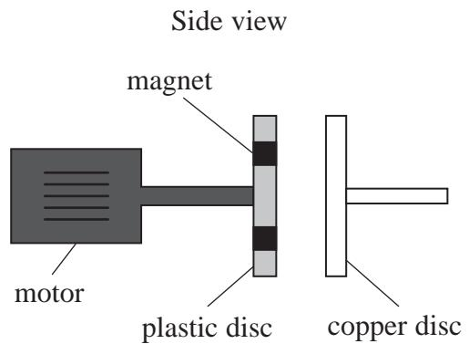
Several magnets are embedded in the plastic disc and it is rotated by the motor.
